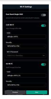
Dual-Band Single SSID: After this feature is enabled, the 2.4 GHz SSID will be consistent with the 5 GHz SSID and the 5 GHz band will be preferred. The 2.4 GHz signal is strong but easily interfered by various wireless signals. The 5 GHz band boasts fast speed, low latency and less interference.
